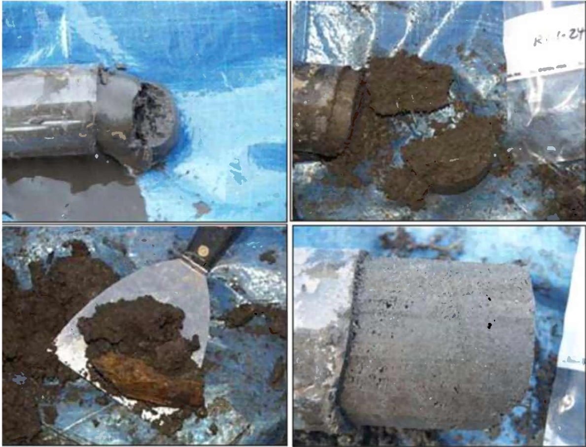
Figure 12. (a) Upper left shows sediment from the top of Core 1, illustrating its fine, organic texture and lack of cohesiveness. (b) Upper right shows large piece of woody debris at 95 cm. (c) Lower left shows small, numerous pieces of vegetation and larger woody debris and comparatively low water content. (d) Lower right shows bottom of core with higher sand content.
